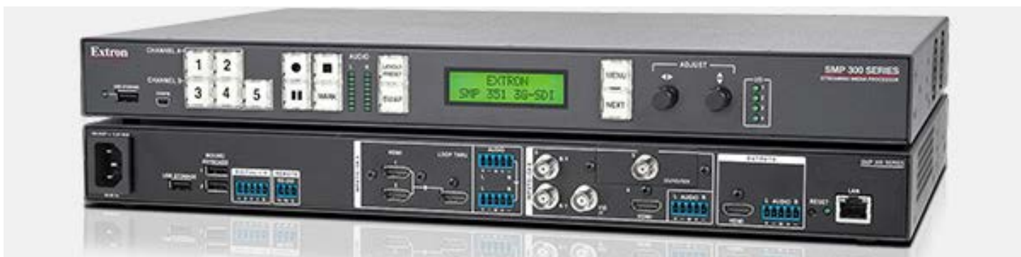
Extron SMP300 multi-channel H.264 streaming media processor
